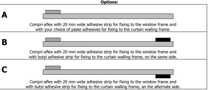
For membrane widths over 150 mm and when using the versions with butyl rubber adhesive tape: it is necessary to apply an additional mechanical fixing or an additional sticking with Compri-fen adhesive (on walls).
